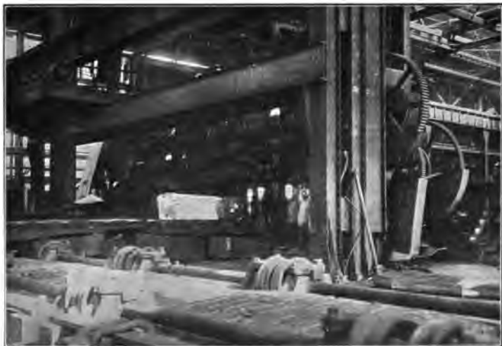
FIG. 118.—Steel ingot about to enter rolls.
